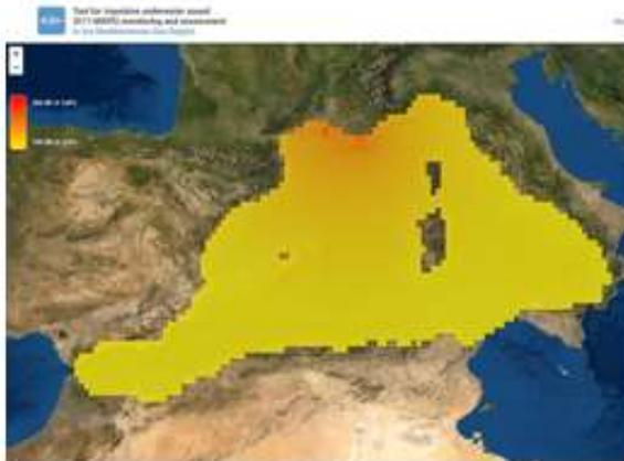
**Pressure maps** are generated from the information included in the INR-Med section by applying acoustic modelling.
